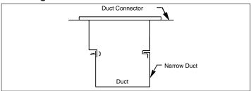
Figure 11. Narrow Duct Installation
